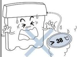
If the inlet water temperature is over 38°C, it will damage the reverse osmosis membrane leading to membrane failure.
