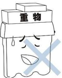
If heavy objects are placed on the water purifier, it may result in damage to the water purifier's dust cover or internal components, which could lead to leakage, the machine working improperly, or even serious property damage.
