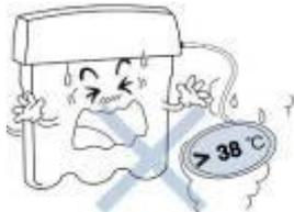
If the inlet water temperature is over 38°C, it will damage the reverse osmosis membrane leading to membrane failure.
