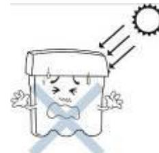
When the water purifier is in sunlight for a period of time, it may create a breeding ground for microorganisms so the water purifier water quality will decrease, and they may pollute the internal components of the water purifier.
