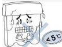
If the temperature in the room is below 5°C, please be sure to take measures to prevent freezing, such as starting the heater or air conditioner to prevent leakage or cracked pipes caused from water freezing inside the machine.
