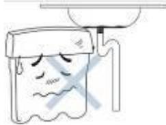
If it is used while the sewer is blocked, it may cause the waste water to back up or pollution to get inside the water purifier.
