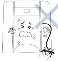
When the waste water discharge pipes and waste water ratio device are clogged, it may lead to high TDS effluent, the RO membrane may get blocked or the water purifier may not work.
