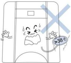
If the inlet water temperature is over 38°C, it will damage the reverse osmosis membrane leading to membrane failure.
