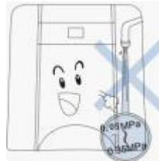
Operating under high-pressure conditions may cause the water purifier pipes to rupture, resulting in leakage, the machine working improperly, or even serious property damage. Recommended inlet pressure is
