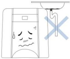
If it is used while the sewer is blocked, it may cause the waste water to back up or pollution to get inside the water purifier.
