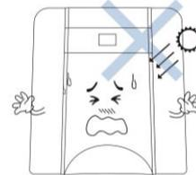
When the water purifier is in sunlight for a period of time, it may create a breeding ground for microorganisms so the water purifier water quality will decrease, and they may pollute the internal components of the water purifier.
