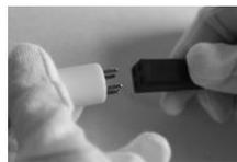
**Step 7:** Hand-screw Closed End Nut on the Reactor Chamber (closed end of Quartz Tube). To protect the O-ring, do not over tighten.
