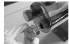
**Step 10:** Carefully insert the UV Lamp into the Quartz Tube through Open End Nut.
